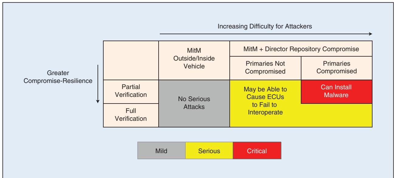
**FIGURE 5** A rough security analysis of Uptane, depending on which repositories and ECUs have been compromised [38], [39]. MiTM: Man-in-the-Middle.
