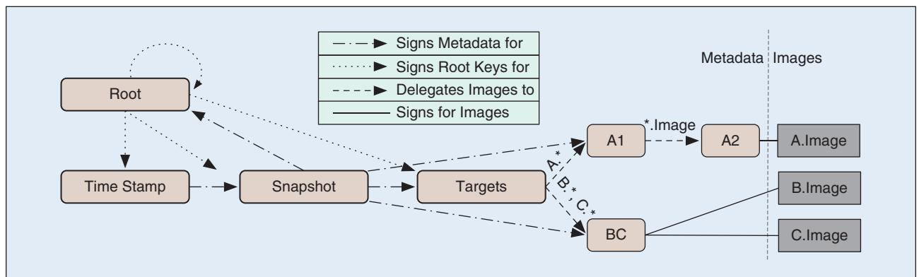
**FIGURE 2** The separation of duties between signing metadata roles [38], [39].
