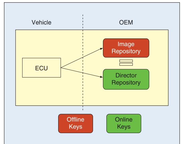
**FIGURE 4** Uptane uses two repositories to provide OEMs with both security and customizability [38], [39].
